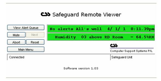
Under normal operation this web interface provides the analogue sensor readings at each update of screen.
